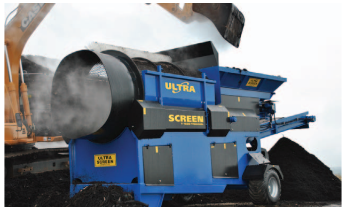
3.5 Cubic Tonne variable speed Feed Hopper, spill plates optional
